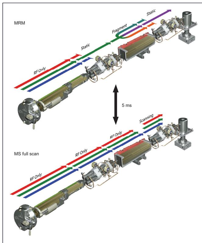
Figure 1. Xevo TQD ion path showing MRM and MS full scan mode acquisition.
